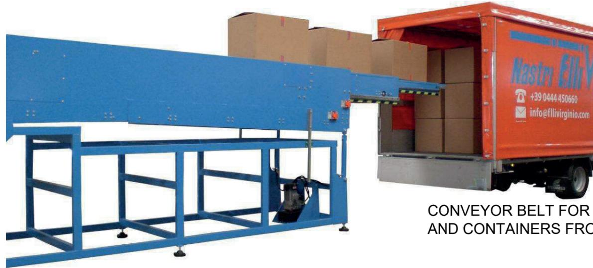
CONVEYOR BELT FOR LOADING TRUCK AND CONTAINERS FROM LOADING BAY
