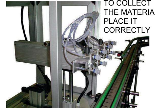
CONVEYOR BELT WITH ROBOTIC HAND TO COLLECT THE MATERIAL AND PLACE IT CORRECTLY
