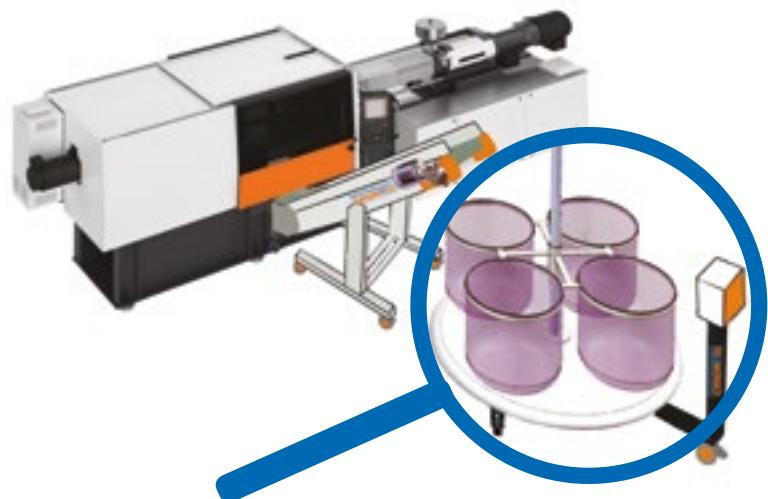
Rotary loading system manufactured in galvanized steel for automatic loading of moulded pieces in boxes or bags. Equipped with control box to manage the rotation with external signal interface from the machine (robot) or independent. Maximum number of boxes/bags 12.
