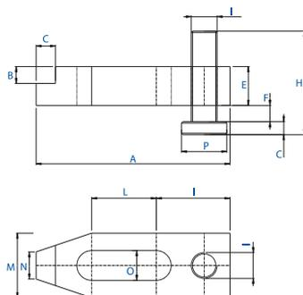
Tempered steel clamps with sliding cables or threaded holes for fixing the moulds to the machine. Thanks to their well-proportioned dimensions, they ensure the indeformability even with heavy loads and prolonged stress.
